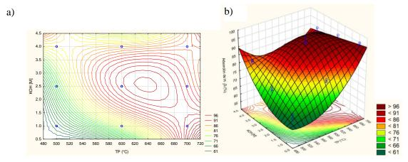
Fig. 2. Simulation of H<sub>2</sub>S adsorption optimization by contour plot (a) and response surface (b)
