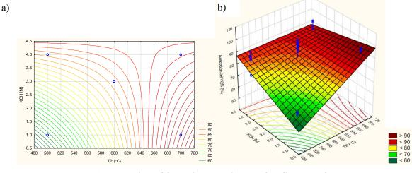
Fig. 1. Design of factorial experiment of H<sub>2</sub>S adsorption by contour plot (a) and response surface (b)
